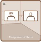
To ensure optimal spray pattern, remove any adhesive buildup that may occur during the application process.
