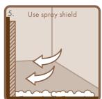
• Protect from overspray with a spray shield, drop cloths, paper, or masking.
